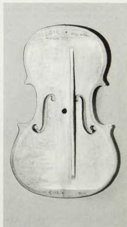
UNDERSIDE VIEW of a violin top plate. The blob of sealing wax at the exact center marks the position that the transducer coil would occupy during a test. The bass bar, a strip of wood glued to the plate, runs under the string of lowest pitch and is therefore off-center. It acts as a stiffening member for the plate and its final shaping is very important in determining the tone of the completed instrument. —FIG. 5
