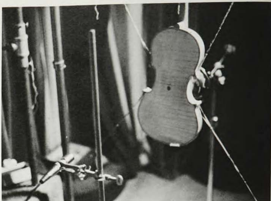
VIOLIN ON TEST RACK. Microphone is in clamp at left foreground; coil that couples audio-oscillator output to instrument is hidden in this view. —FIG. 2
