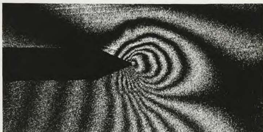
HOLOGRAPHIC INTERFEROMETRY. Fringes in a hologram image of a notched metal bar under stress. The pattern indicates there is plastic flow near the notch.
