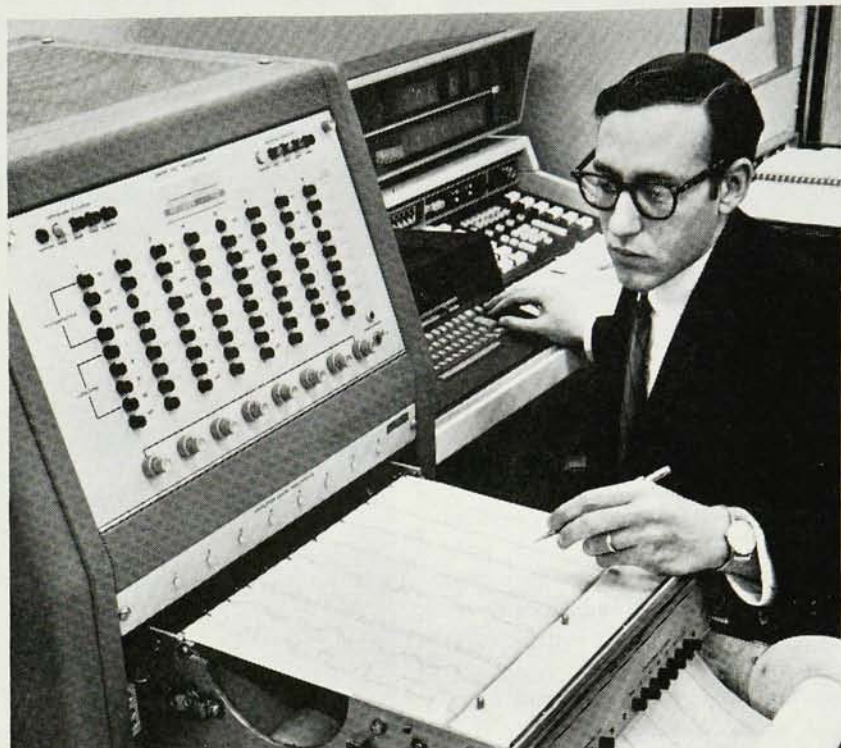
Scientist Barry J. Karafin of Bell Laboratories checks chart recorder waveforms from a BLODIB simulation. Karafin uses the computer console at his right to interact with the simulation program. This feature was developed for the BLODIB program to give users the flexibility of making changes in such things as component values without having to re-program an entire system.
