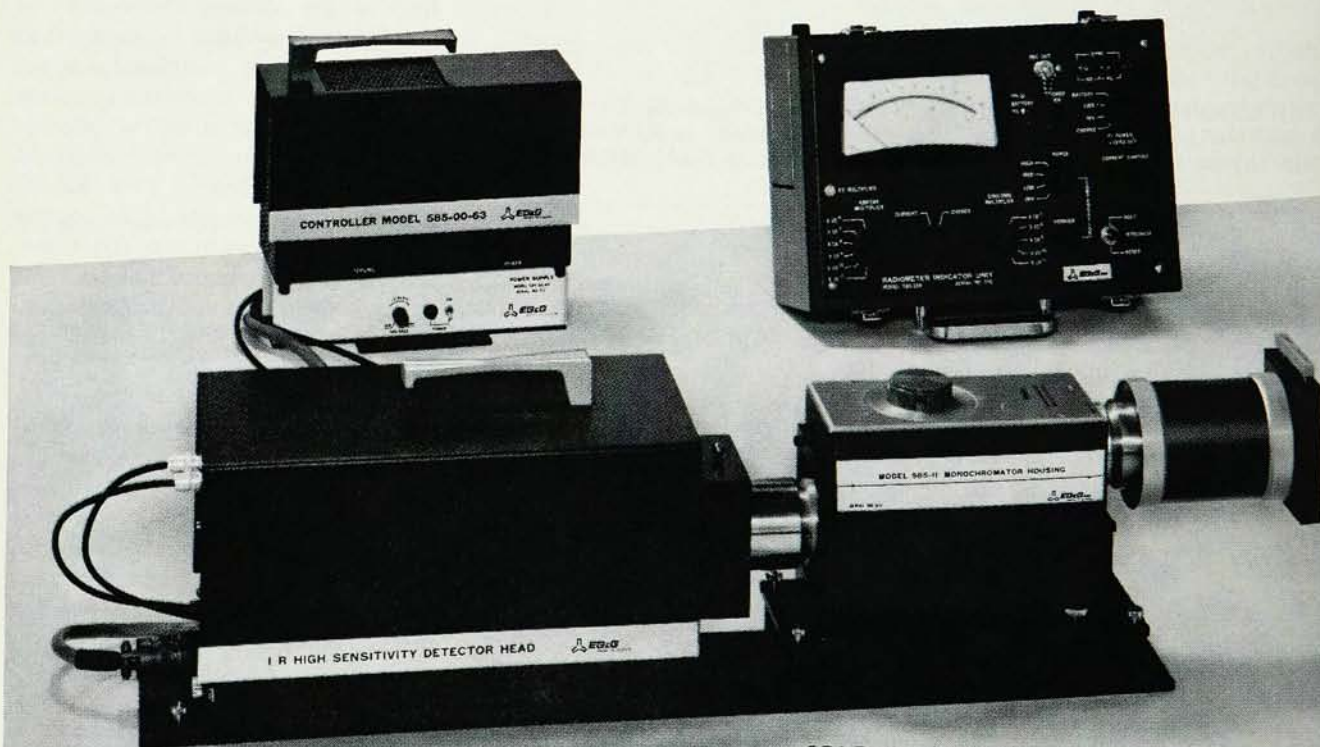
EG&G's Model 580/585 Spectroradiometer features a new IR detector head which is thermoelectrically cooled to minimize thermionic dark current.
