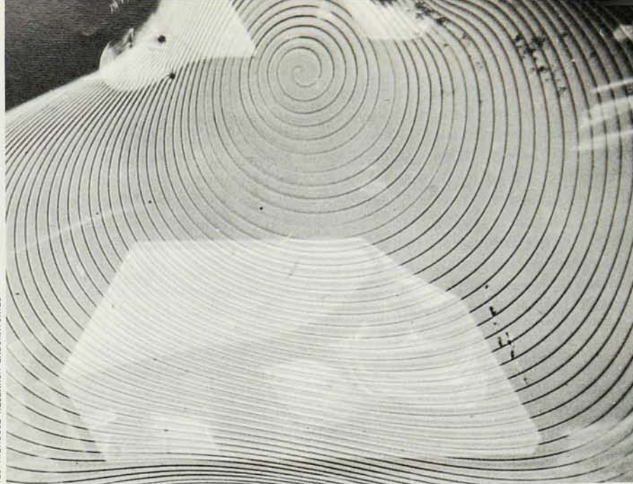
SCREW DISLOCATION AND GROWTH SPIRAL in transparent silicon carbide. As crystal grows, the atoms form a spiral of constant step height, six molecules high.
