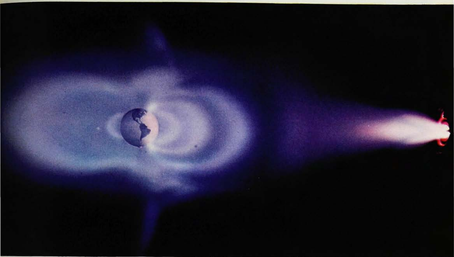
SIMULATION OF THE SOLAR WIND interacting with the earth's magnetic field. This picture was made at the NASA Lewis Research Center, Cleveland, Ohio, in a 4.6 \times 20 -meter vacuum chamber with a magnetoplasmadynamic thruster (right) standing in for the sun. Thrusters such as this one being studied at Lewis have produced exhaust velocities of nearly 48 km/sec. Radiation belts are to scale.
