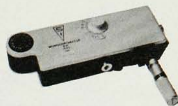
MONOCHROMATOR , miniature quartz prism type, F/7.6 Range 190-1500 mu. Slits are adjustable in unison.
