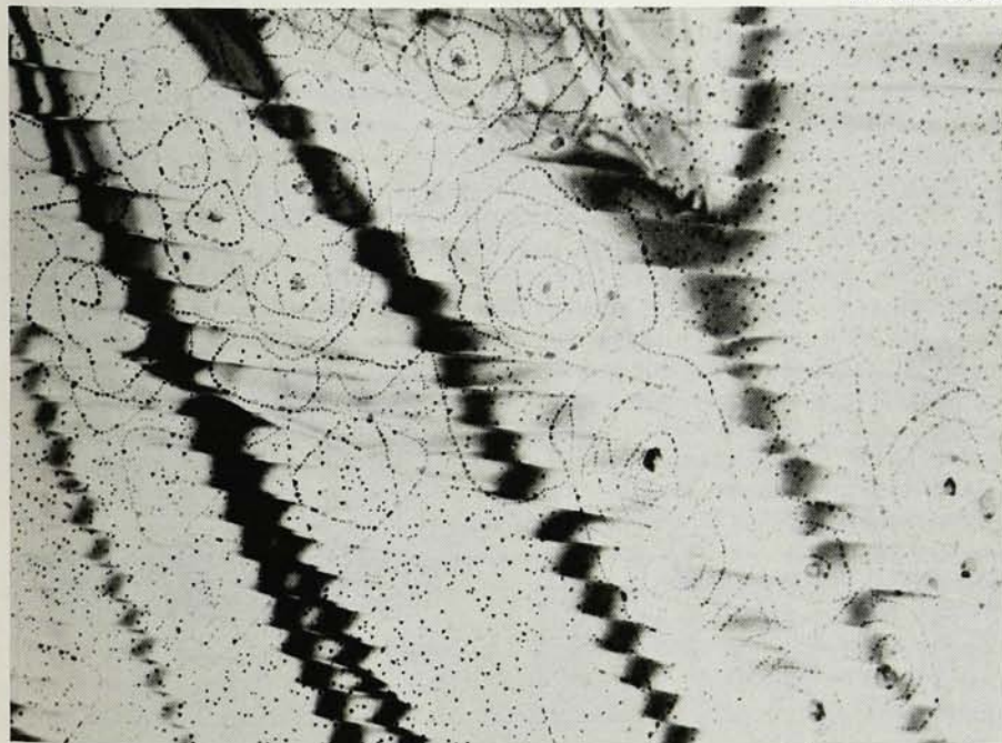
LATTICE VACANCIES IN MOLYBDENITE are revealed by etch decoration. Gold atoms nucleate at vacancies, which show up on electron photomicrograph. Centers of the small triangular depressions appear to correspond to surface vacancies.
