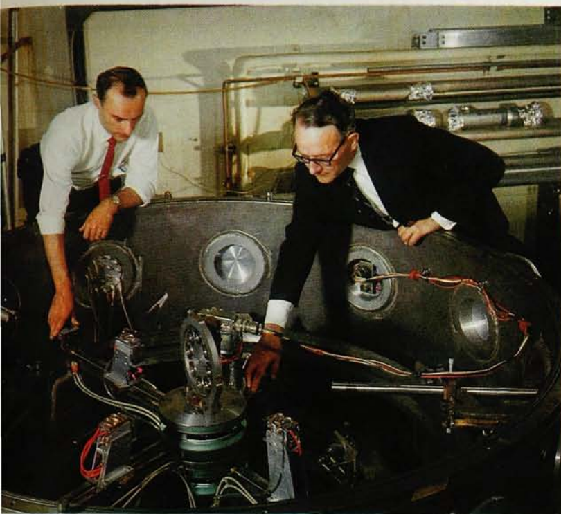
152-CM HIGH-PRECISION SCATTERING CHAMBER used at Argonne 18-MeV tandem. Computer controls detector positions, makes decisions.
