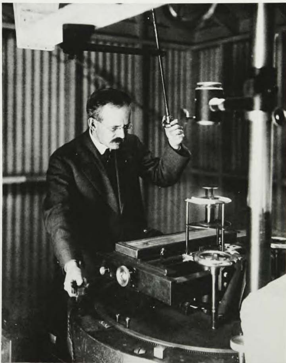
GEORGE ELLERY HALE using his spectroheliograph. The instrument records solar flares photographically. (Courtesy of Mount Wilson and Palomar Observatories).
