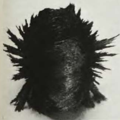
PERMANENT MAGNET suitable for small dc motor. Modern materials contribute to component miniaturization.
