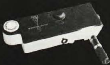
MONOCHROMATOR , miniature quartz prism type, F/7.6 Range 190-1500 mμ. Slits are adjustable in unison.
