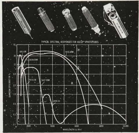
The unusually wide selection of photocathodes and window materials offered in EMR multiplier phototubes permits tailoring a special response characteristic to virtually any spectral region of interest. These characteristics, coupled with extreme resistance to hostile environmental conditions, have created a unique place for them in fields as diverse as deep space spectrometry and geophysical research.
