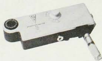
MONOCHROMATOR , miniature quartz prism type, F/ .6 Range 190-1500 mμ. Slits are adjustable in unison.
