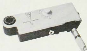
MONOCHROMATOR , miniature quartz prism type, F/ .6 Range 190-1500 mμ. Slits are adjustable in unison.
