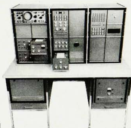
ND-520PAD Preamplifier, Amplifier, Discriminator; ND-534LARC Linear Amplifier; ND-535DS Decade Scaler; ND-530ID Integral Discriminator; ND-539TM Timing Meter; ND-536CTB Clock/Time Base; ND-537HVS High Voltage Supply.
