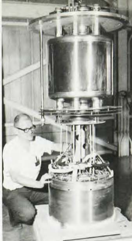
140-kG SUPERMAGNET. Above magnet proper is the dewar-lid assembly.
