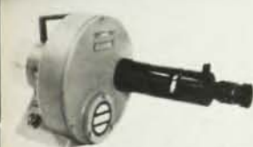
SUPER DYNAFAX MODEL 318 streak camera records at rates up to 0.306mm per microsecond with time resolution of 1.8 \times 10^{-7} seconds.
