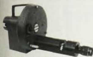
DYNAFAX MODEL 351 streak camera records at rates up to 0.13mm per microsecond with time resolution of 0.4 \times 10^{-6}
