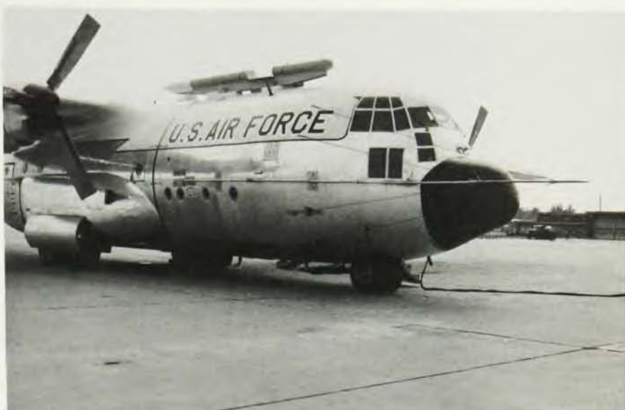
INSTRUMENTED AIRCRAFT can quickly transport heavy instruments. This aircraft is equipped for atmospheric optics research. —FIG. 2
