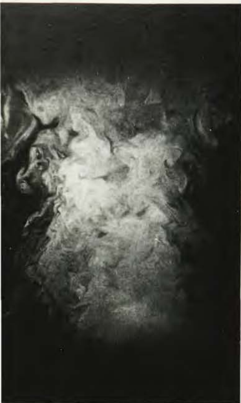
SUBSONIC SMOKE JET seen in the planar light from an ultraviolet nitrogen laser operated in short-pulse mode with peak power of 100 kW. —FIG. 2
