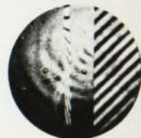
EVALUATION OF INSULATION MATERIALS BY MEASURING FRINGE PATTERN IN AIR GAP.
