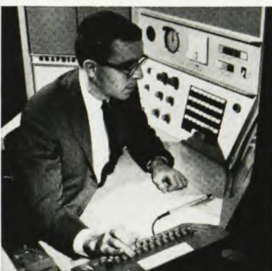
4. With a keyboard, which resembles a typewriter, he inserts the values of the various components and the operating conditions of the circuit.
