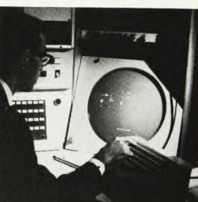
6. Seeing the curve, he may modify the circuit, insert new values for variable components, request the computer to recalculate performance.
