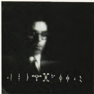
1. A program for GRAPHIC I lets engineer W. H. Ninke draw a circuit diagram on a cathode ray tube, using familiar component symbols.
