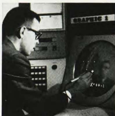
2. In describing a circuit problem to the computer, he guides nodes (circuit junction points) into place with a light pen.
