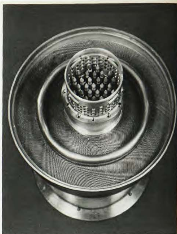
FUEL ELEMENT of the HFIR is shown at right with target rods in the central trap. To reduce "hot spots" the fuel elements are graded as shown in the schematic of the fuel-element cross section shown at left. —FIG. 3
