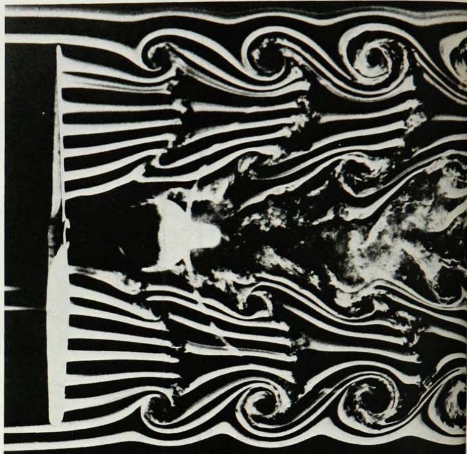
TURBULENCE in the wake of a propeller made visible by streams of smoke injected into the backwash of the propeller. Instead of smooth flow we have all kinds of vortex motion appearing.
