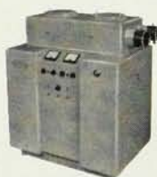
Model 225 — 1 meter normal incidence vacuum scanning monochromator McPherson type. Range 300A — 6,000A.
