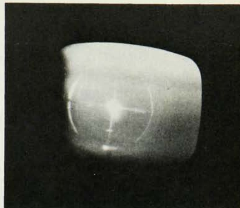
BEAM SPOT as observed at end of two-mile accelerator. —FIG. 16
