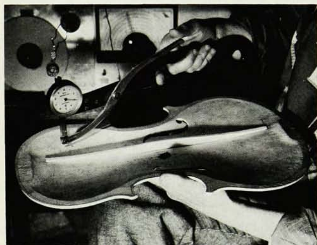
TESTING FIDDLES. New techniques enable today's makers to achieve results their predecessors could not produce. Redesigned transducer measures response of plate that is made to vibrate like a loudspeaker cone in operation. —FIG. 6
