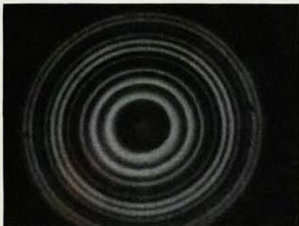
Operated with fixed spacing, 6328A laser modes are resolved in this classical image display.
