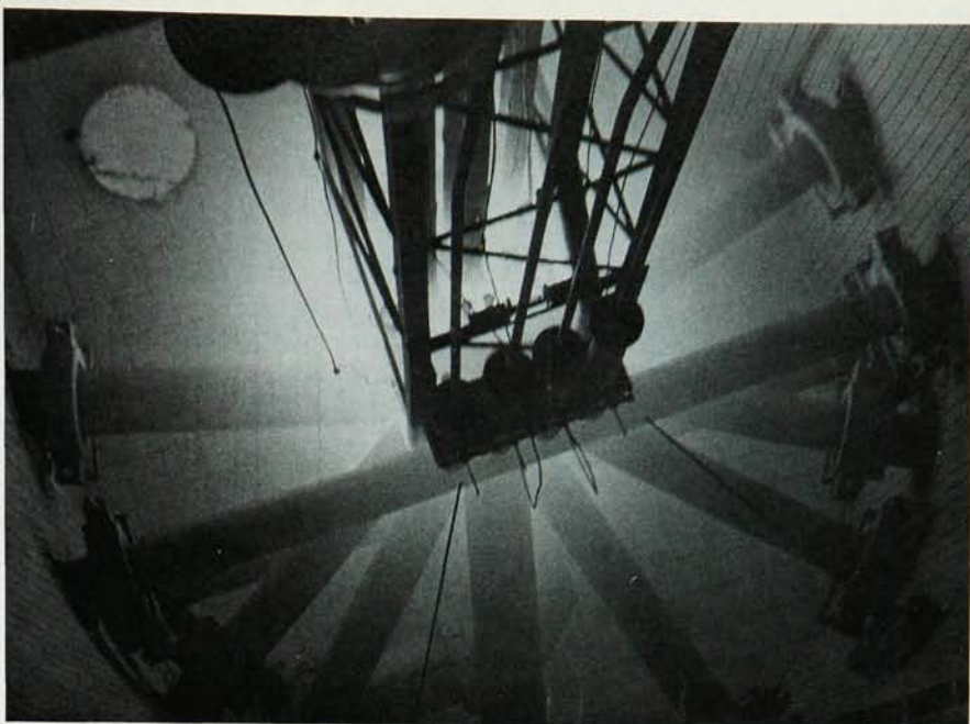
CERENKOV RADIATION as seen coming from the U. of Michigan reactor.
