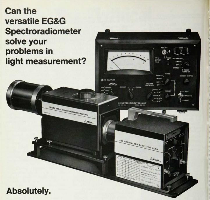
For scientists, the versatility of the EG&G 580/585 Spectroradiometer has made it the ideal system for many different applications. It can measure continuous and pulsed light sources as fast as 1 nsec, with a spectral range from 200 to 1200 m $\mu$ , over six decades of incident light energy and power. The 580/585 can perform absolute spectral measurements, with direct meter or recorder output, of:
