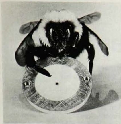
INFRARED DETECTOR (tiny black spot in center of white circle), dwarfed by eye of accompanying bee, is being used to analyze radiation from the earth's horizon.
