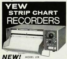
Self-folding chart stacks flat! Data easily scanned and stored. Solid state. Potentiometric; single turn slide wire. Up to 17 self-contained ranges from 1 mV-100 V. Chart speeds 2/6/20 cm/min and cm/hr; combs. available from 40 cm/min. Dead band  $\pm 0.1\%$  fs. Accuracy to  $\pm 0.25$  fs. Portable or rack mounting.
