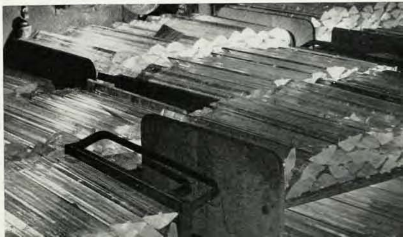
Rochelle salt crystals ready for machining The Brush Development Company
