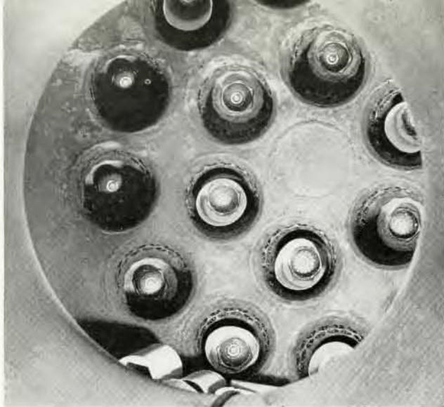
Looking into the throat of a V-2 motor and showing paper collars used to prevent incorrect oxygen impingement at start of flow.
