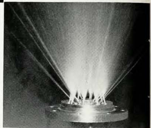
Water test showing manner in which fuel and oxidizer impinge in a liquid propellant rocket.
