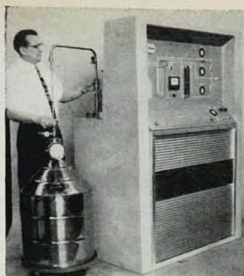
CRYODYNE® Helium Liquefier and Refrigerator. This compact, semi-automatic device can produce up to 70 liters a week of liquid helium and can also be used as a 4.2°K closed-cycle refrigerator.
