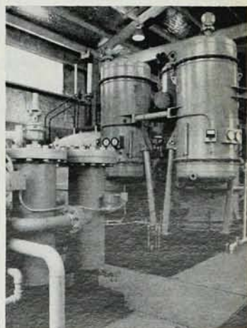
ADL MULTIPOD Helium Plants. For large-scale production of liquid helium or as major sources of helium-gas refrigeration, these plants are available in six models. Liquefaction capacities from 35 to 120 liters per hour; refrigeration capacities from 750 to 2,000 watts at 20°K, 200 to 400 watts at 4.2°K.
