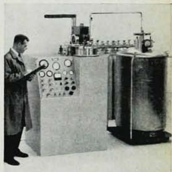
ADL MULTIPOD Helium Plants. For large-scale production of liquid helium or as major sources of helium-gas refrigeration, these plants are available in six models. Liquefaction capacities from 35 to 120 liters per hour; refrigeration capacities from 750 to 2,000 watts at 20°K, 200 to 400 watts at 4.2°K.
