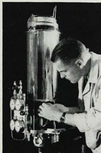
ADL CRYODYNE® Maser Refrigerator. For use in global and space communications systems, this reliable system can provide 1.0 watt of refrigeration at 4.2°K and will run continuously for 3,000 hours before preventive maintenance is required.
