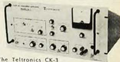
The Teltronics CK-3 Lock-In Converter Amplifier . . . a universal narrow-band signal processor which utilizes the technique of synchronous detection for recovery of signals buried in noise.
