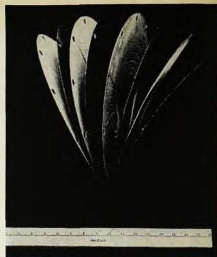
BITTER MAGNET PLATES and insulators. Dark plates are copper and are arranged to form a continuous helix. Light plates are insulators. Cooling water goes through axial holes.
