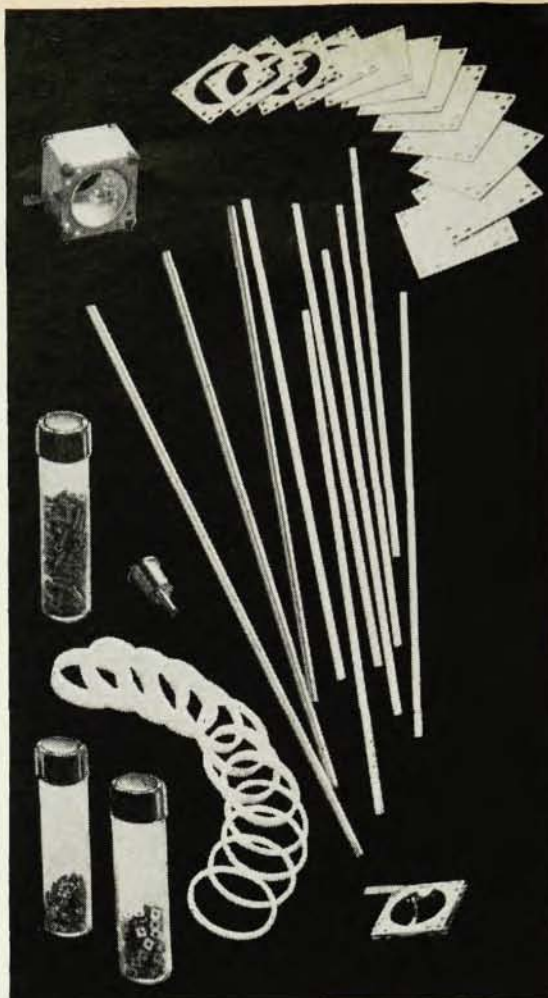
BITTER MAGNET PLATES and insulators. Dark plates are copper and are arranged to form a continuous helix. Light plates are insulators. Cooling water goes through axial holes.
