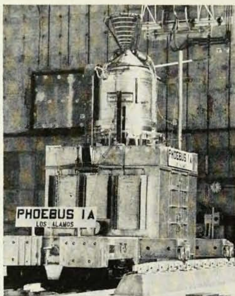
PHOEBUS 1A , a 1000-MW nuclear-propulsion reactor, at LASL's nuclear-rocket development station in Nevada.
