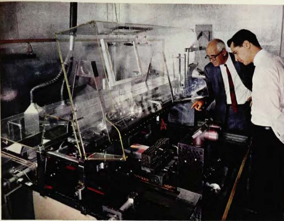
In the Spectroscopy Laboratory at MIT, Dean George R. Harrison and Stephen W. Thompson inspect interferometrically controlled ruling engine.
