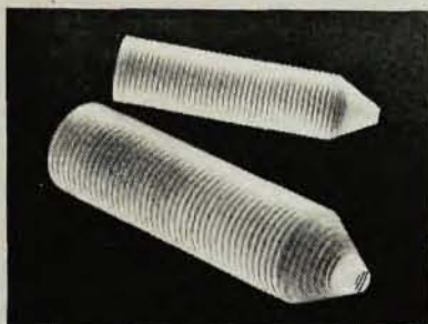
This unique 3.5" cylinder with .475 \pm .001 " conical taper and 1/32 " spiral groove has ends flat to 1/20 th wave and parallel to 2 seconds of arc.
