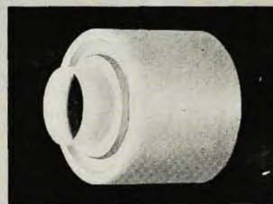
Fabricated from high quality optical fused silica, this viewing window-flat is used as a photographic window in tunnel applications. The unit has a 5" diameter and 10" diameter both of which are flat to 1/10 th wave of sodium light.
