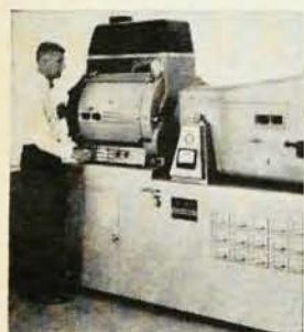
ADL-Strong Arc Imaging Furnace A general-purpose high-temperature furnace for laboratory use.
