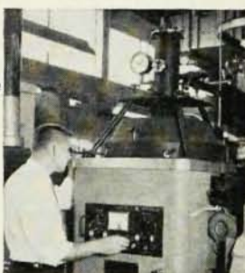
ADL-Strong Arc Imaging Furnace A general-purpose high-temperature furnace for laboratory use.
