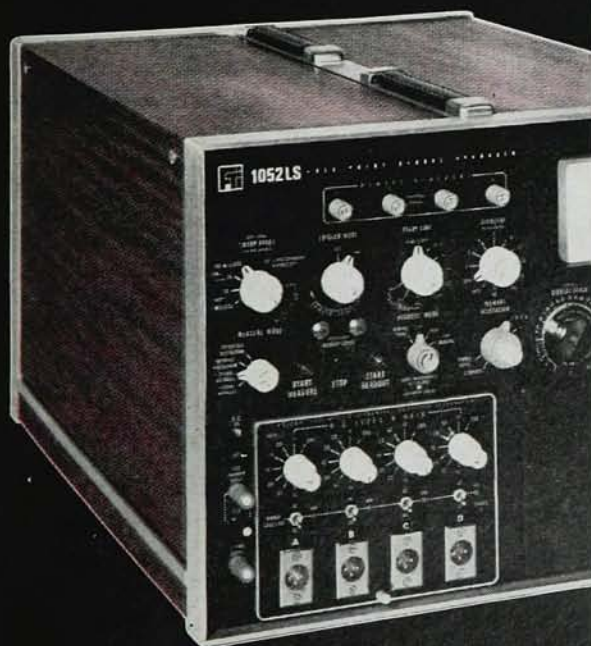
FT-1052LS 1024 word memory averager with FT-100 4 input amplifier/integrator
