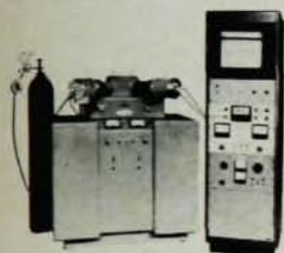
MODEL 235 Half Meter Scanning Monochromator, Seya-Namioka Range 300—6,000A
