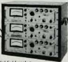
Triaxial Magnetometer System Model MF-55-331
