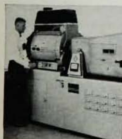
ADL-Strong Arc Imaging Furnace A general-purpose high-temperature furnace for laboratory use.
