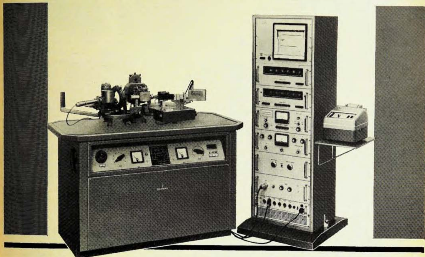
KRISTALLOFLEX IV with polefigure-goniometer and powder diffractometer
