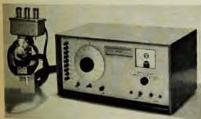
CEC 21-612 RESIDUAL GAS ANALYZER
