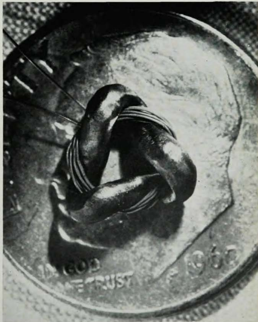
Fig. 1. First stage in building Furth-Rosenbluth "snake wrapped around a pole" (tuning coil around indium-antimonide crystal)
