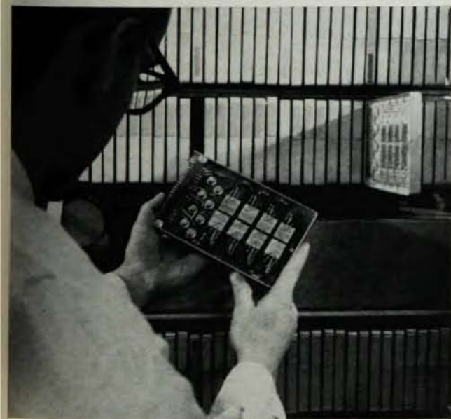
Experimental automatic data equalizer devised at Bell Laboratories. Control section consists of the circuit packages; the package being inspected is one of 12 attenuators, the settings of which determine the degree of distortion-correction of the equalizer.
