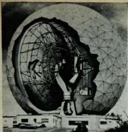
Cut-away drawing shows Haystack antenna in its protective radome. One of three "plug-in" boxes carrying experimental gear is being hoisted up behind antenna.
