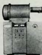
1 METER NORMAL INCIDENCE SCANNING MONOCHROMATOR ROWLAND CIRCLE, RANGE 300Å - 6,000Å*
