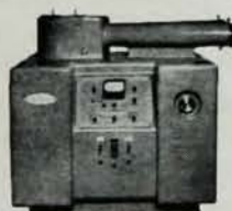
1 METER SCANNING MONOCHROMATOR SEIYA-NAMIOOKA RANGE 300Å - 6,000Å*
