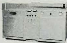
2 METER COMBINATION SPECTROGRAPH AND SCANNING MONOCHROMATOR, EAGLE RANGE 300Å - 6,800Å*
